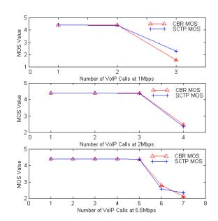
Figure 4 CBR and SCTP MOS for G.711 at different data rates
