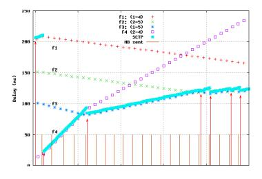
Figure 17 Delays on forward path with SCTP bandwidth increase (packet size=100, interval=0.2 s). Vertical lines at the bottom indicate when HB probes were sent. Vertical arrows indicate when transmission is switched to a new path with lower delay. At t=38 s SCTP switches back and forth between paths  $f_2$  and  $f_4$  due to self traffic loading on current selected path.
