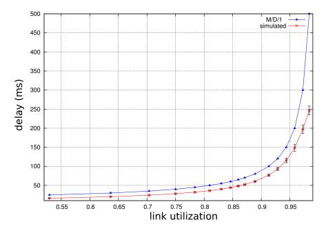
Figure 7 Averaged delay versus system utilization
