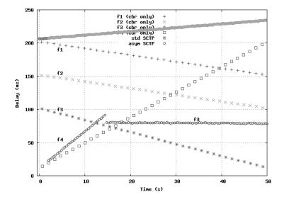
Figure 16 Comparison between: (1) standard SCTP (primary path only:  $f_1$ ); (2) Symmetric delay-centric SCTP (primary round-trip path ( $f_1r_1$ ) has the lowest RTT; (3) Asymmetric SCTP (paths  $f_1, f_4, f_3$ ); (4) Delay of CBR background cross traffic (with no SCTP traffic) was also plotted for reference.
