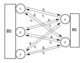
Figure 10 Multi-homing with asymmetric paths. Forward and reverse paths are identified.
