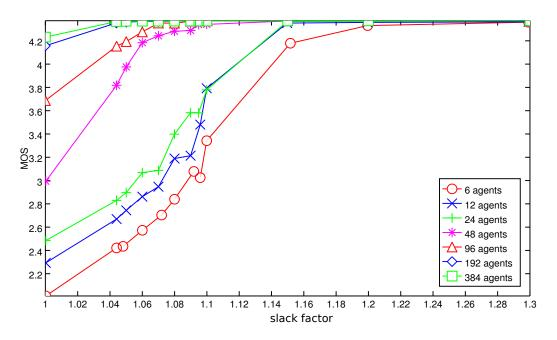
Figure 6 Calculated MOS for different number of competing SCTP transmissions versus slack factor
