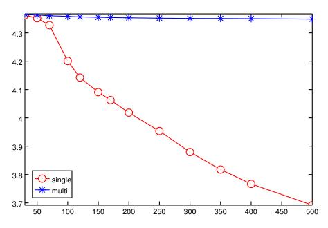
Figure 9 Calculated MOS versus delay for multipath and single path
