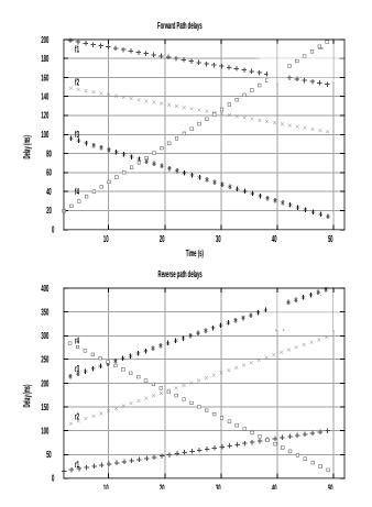
Figure 15 UDP packet delays - CBR traffic only. (a) forward paths. (b) reverse paths.
