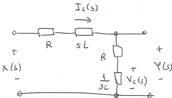
$$\begin{cases} X(s) = R I_L(s) + \underline{sL I_L(s)} + R I_L(s) + V_C(s) \\ \underline{sC V_C(s)} = I_L(s) \\ Y(s) = R I_L(s) + V_C(s) \end{cases}$$
