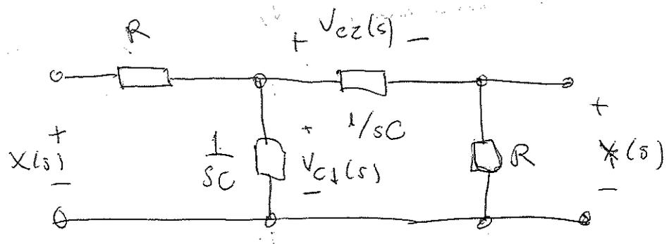
$$sC V_{c2}(s) = \frac{V_{c1}(s) - V_{c2}(s)}{R} = \frac{Y(s)}{R}$$
