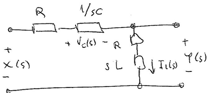
$$X(s) = R I_L(s) + V_C(s) + R I_L(s) + sL I_L(s)$$
